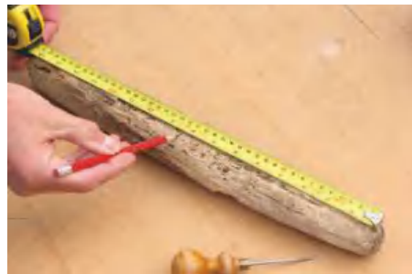
▲ Pic.2 Measure each branch and mark the approximate centre point. This is definitely not fine woodworking!
